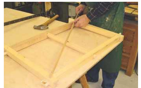
▲ Pic.18 Check the glass panes are the same size; measure the distance between top and bottom rail
